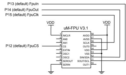
The clock signal is idle low and data is read on the rising edge of the clock (often referred to as SPI Mode 0).
