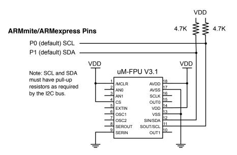
FpuPin Pin 0 (SDA is Pin 0, SCL is Pin 1)
